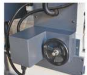
Optional Infeed by Motor Control (0,005mm)
