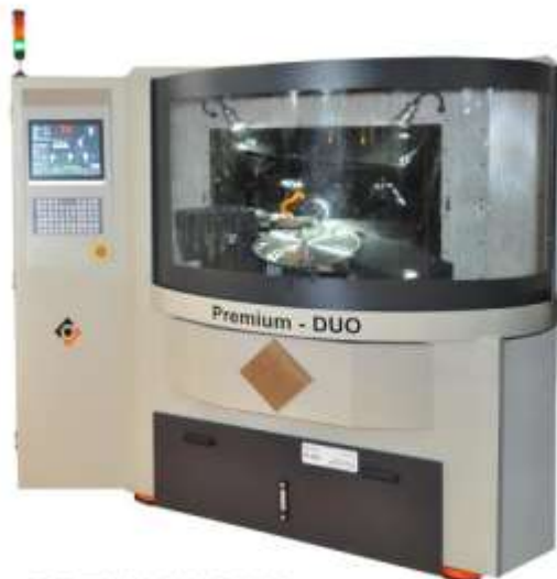
PREMIUM-DUO 8 Axes Double Wheel Complete Side Grinder in One Cycle Slide Grinder 8 Axes Servo Motor - PC Control Automatic Measurement and Tooth Data Recognition Circular Saw Diameter: Ø150-600mm (Optional Ø800mm)
