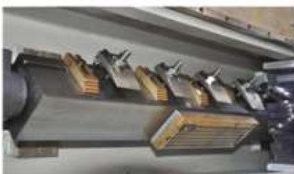
Mechanic Plate with T-Slot System, Optional Reversible-Knife Grinding for Inserts
